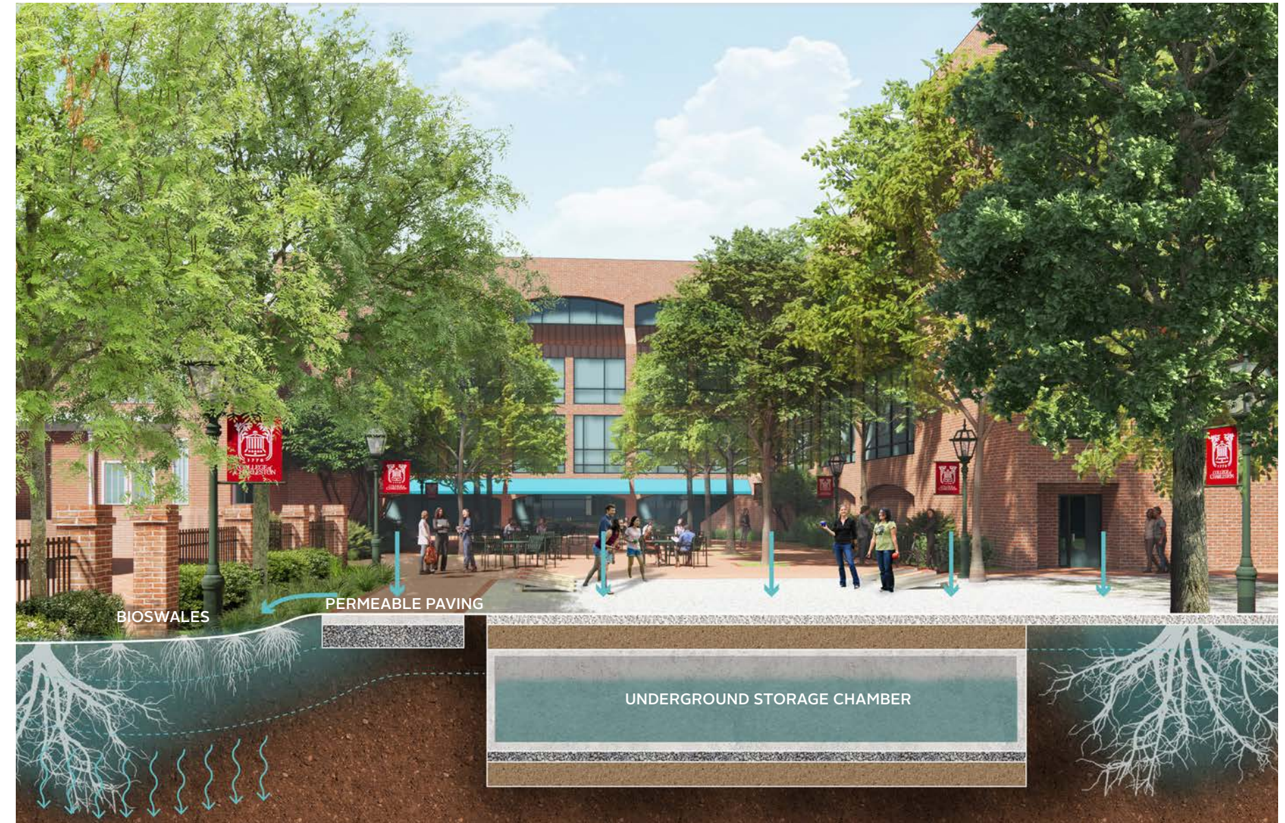
STERN CENTER GARDEN UNDERGROUND STORMWATER STORAGE: To complement the existing opportunities for rainwater harvesting, the Campus Framework Plan recommends incorporating underground storage chambers in all major open space and streetscape improvement projects. For example, the transformation of the Stern Center Garden can incorporate a significant underground storage chamber by partially utilizing the existing sunken courtyard.
